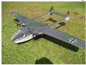
Kaley. It's a Gotha Go 244, from a Jack Bale plan, with an 82"inch wing span and 2 brushless outrunners on a 4s 3000mah. The original plane was built as a glider, for troops and equipment (the Gotha go242) then the Germans found a bunch of radial engines and the 244 was born. We didn't see it fly but next comp ......!
